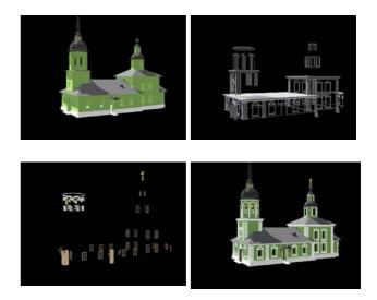
Figure 1: Structured VRML model. Top left: LOD 0, top midright: supplement to LOD 1, down left: supplement to LOD 2, down right: vomplete model containing all three sub-structures.
