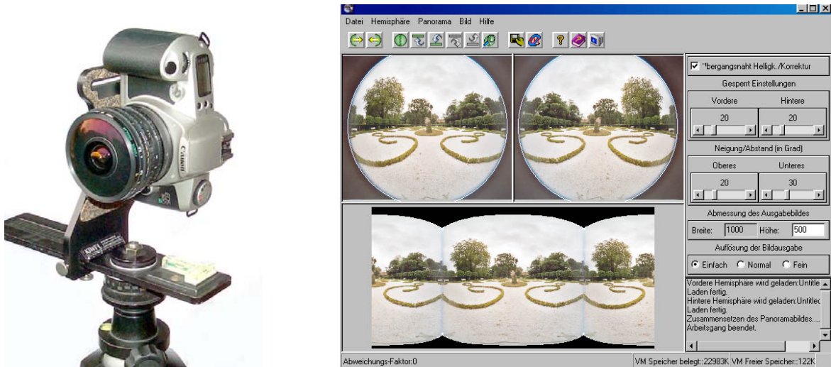
Figure 1: Standard SLR consumer camera with an 8 mm fish eye lens mounted on a panoramic head. Two of those shots with 180-degree different exposure directions can be converted to a full spherical panorama.
